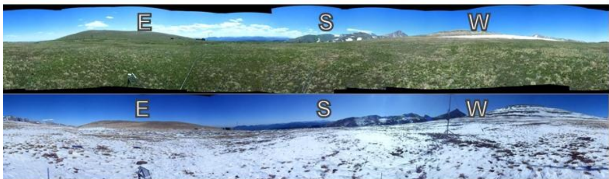
Figure 54: Sky visibility in the 360° surroundings of the GPS antenna at the alpine site (NWOT).
